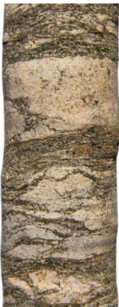
Fig. 1. A borehole core (40 mm diameter) of highly stressed gneiss extracted from great depth in Namibia. It has deformed from its original perfect cylinder as a result of uneven relaxation since being unloaded by being brought to the surface.
